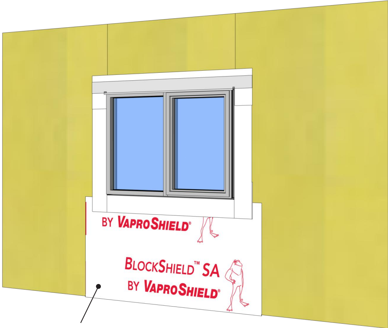
BlockShield SA for Walls field membrane installed underneath 6" flap of VaproFlashing SA to create shingle effect
