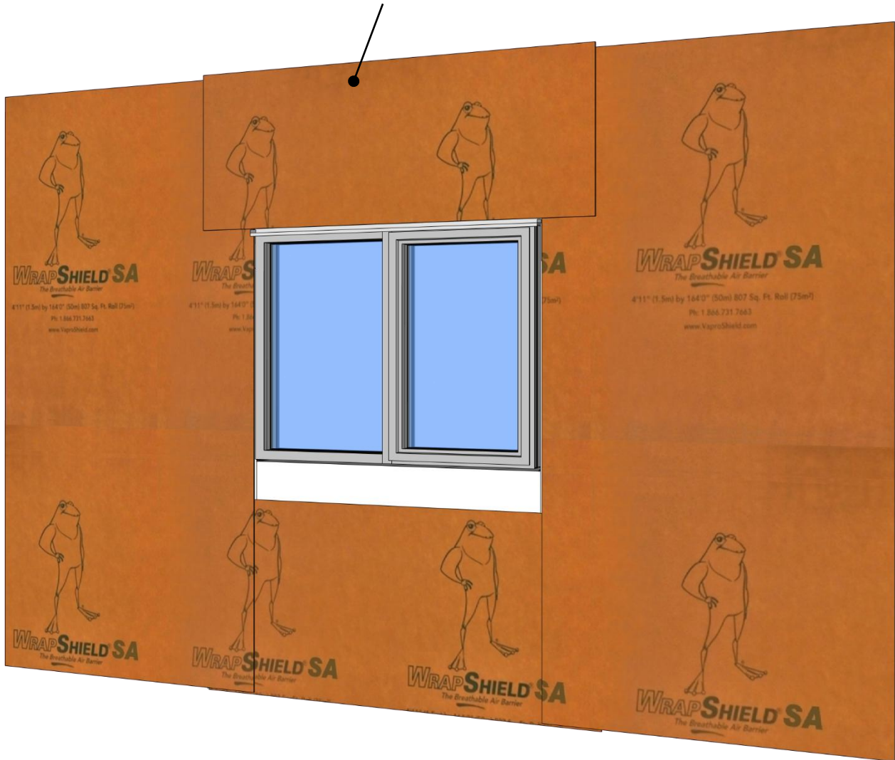
WrapShield SA Self-Adhered installed over head flashing and VaproFlashing SA
